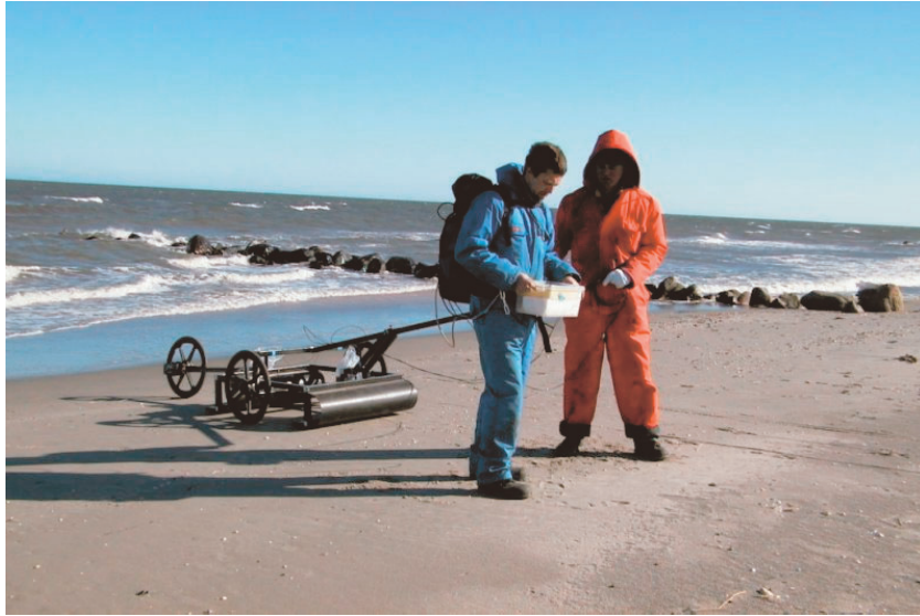
Figure 7. Ground penetrating radar (GPR) measurements performed on shore in the area of known coastal gas seeps south of Frederikshavn.
