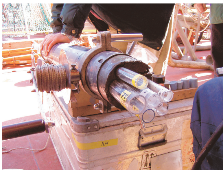
Figure 10. Sub-sampling of the 1-m sections of a gravity core for detailed analyses of geochemical and microbiological parameters and process rate measurements. Core liners of various diameters were pushed from the top into the sediment.
