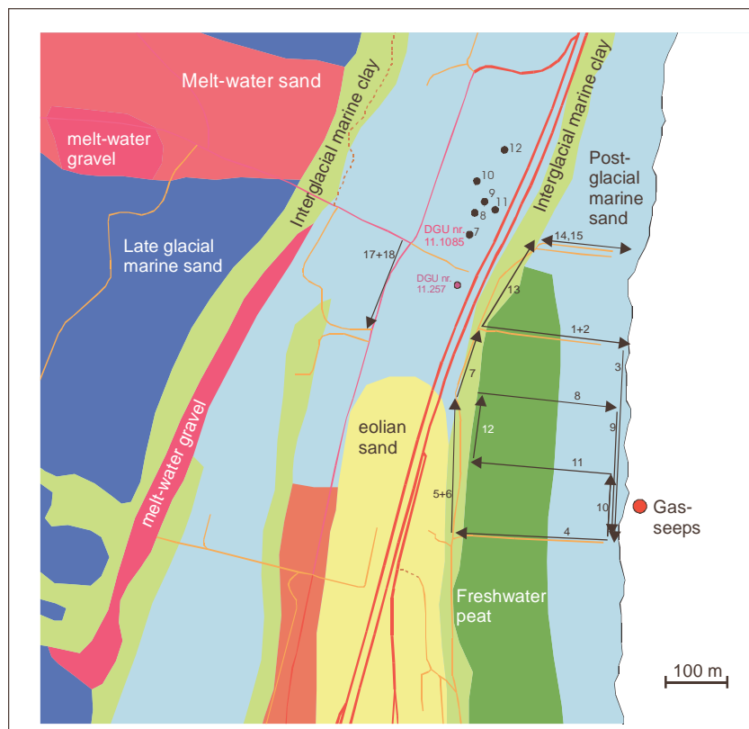
Figure 8. Georadar lines plotted on a sub-surface soil map of the area around the coastal seepage site.
