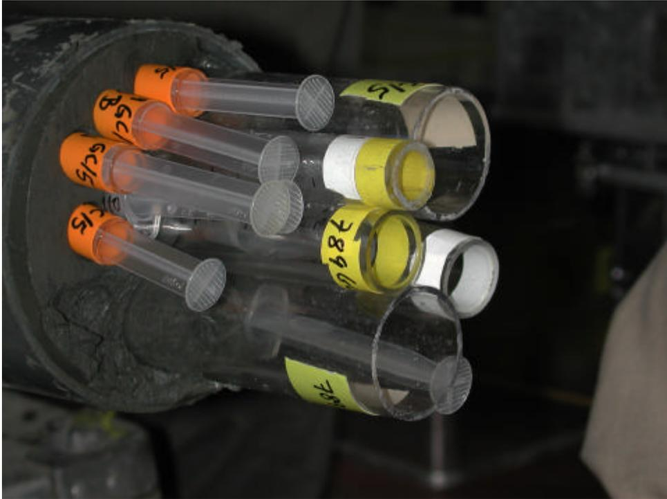
Figure 16. Sub-sampling of the 1-m sections of a gravity core for detailed analyses of geochemical and microbiological parameters and process rate measurements. Core liners of various diameters were pushed from the top into the sediment.
