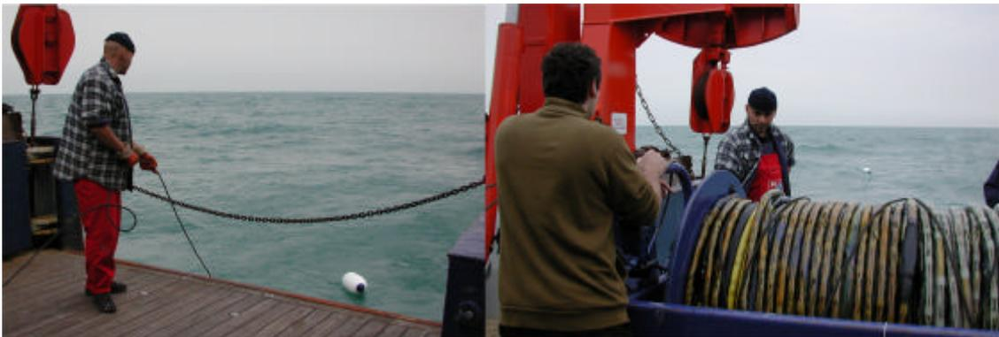
Figure 4. Launching of the streamer
