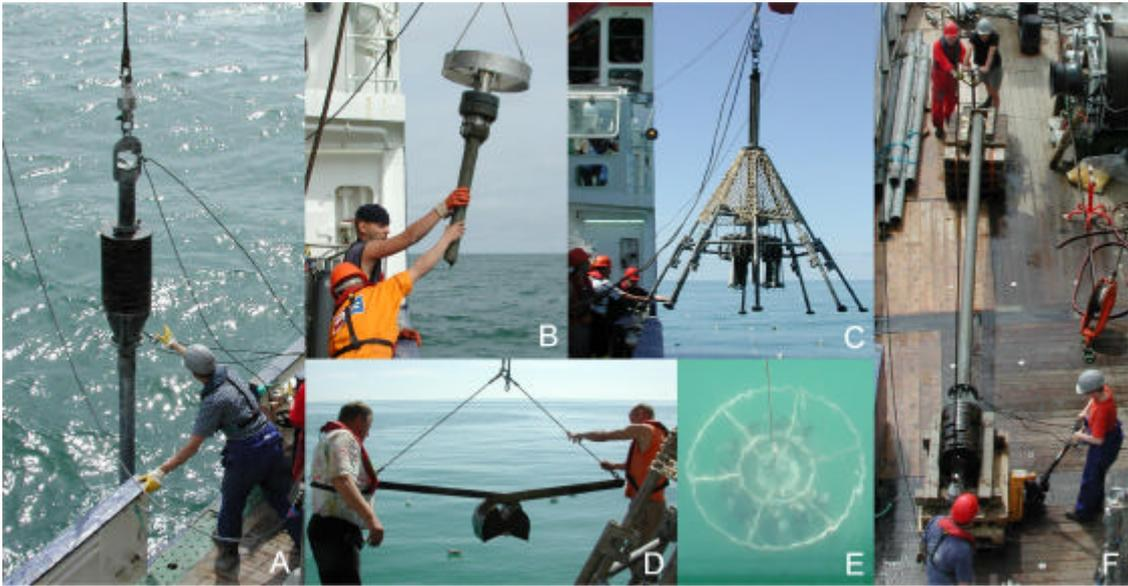
Figure 2. Sampling gear. A: Recovery of the gravity corer. B: Rumohr lot with sediment core visible through the wall of the plexy-glass liner. C: Multi corer filled with 30 cm long cores. D. 0.2 m<sup>2</sup> Van Veen grab. E. The CTD/Rosette just below the water surface on the way down. F: After recovery, the gravity corer is laid down horizontally.
