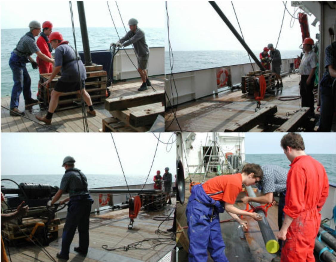
Figure 5. Recovery of the gravity corer and start of core processing.
